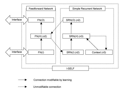
*Figure 1.* A schematic depiction of the I-SELF (Imitative and Sequence Learning Functional) architecture consisting of two functional neural network systems, Feedforward Network (FN) and Simple Recurrent Network (SRN). *Note:* FN stands for Feedforward Network; SRN stands for Simple Recurrent Netwok; I, O, and H in the parentheses indicate input, output, and hidden layers; *n*1, *n*2, and *n*3 stand for the numbers of units in each layer.
